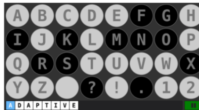
Figure 1: Virtual keyboard. If the bit in the corresponding binary stimulation sequence is 0 the character flickers in light grey, if it is 1 in black.
