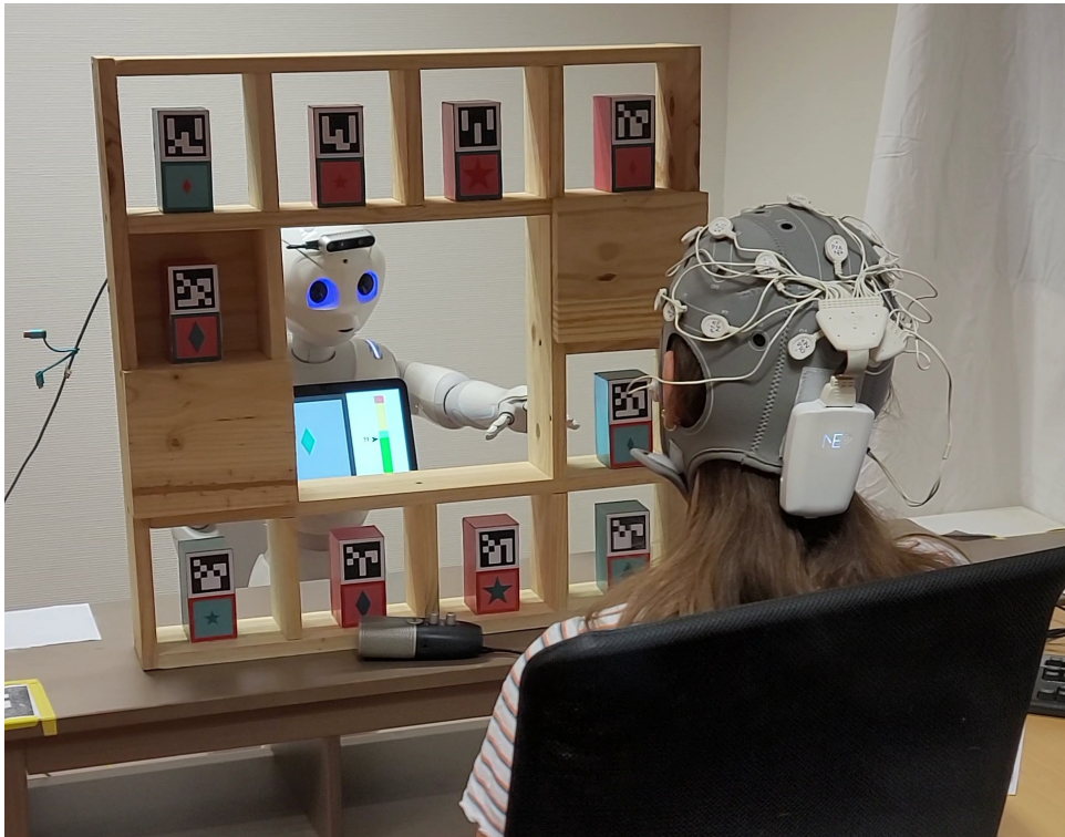
Figure 1: Experimental setup showing the participant equipped with the EEG system, interacting with the Pepper robot through the cube grid task.
